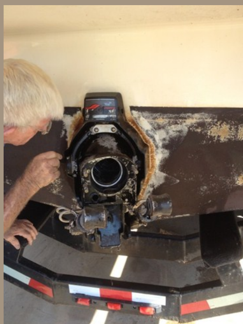
Fig. 2 – Pete Hilton, owner of Quality Marine Service, cleans and de-contaminates this vessel after Zebra Mussels were found on the engine mount.
